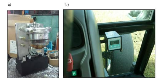
Figure 1. Measurement unit a - flow meter ZP@-4-1 by Rotameter company, b - NOSAL-TECH mounted on a tractor
