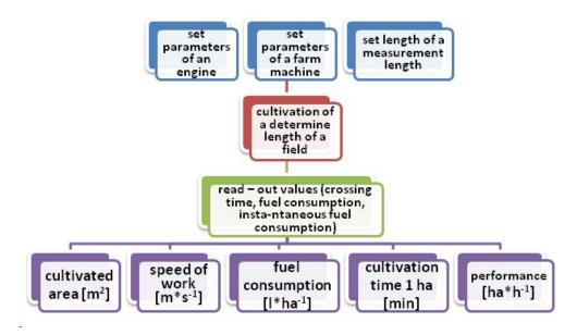
Figure 2. Schematic representation of procedure during exploitation tests
