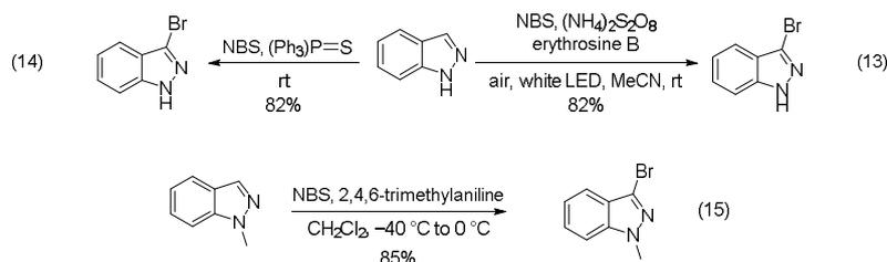
**Scheme 5.** Bromination at the 3-position in the presence of NBS in various conditions.
