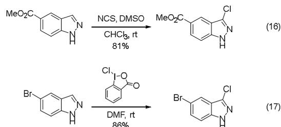
**Scheme 6.** Chlorination at the indazole 3-position using various conditions.
