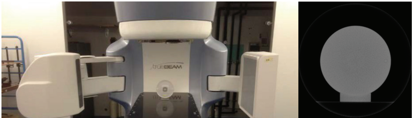
FIGURE 4.3.2. Left: An example of the DIN phantom for constancy tests (QUART DVTkp) placed in a TrueBeam Varian linear accelerator (left) and the acquired image of the uniformity module of the phantom (right).
