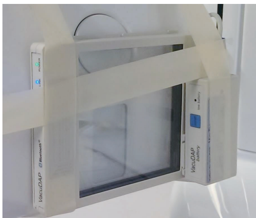
FIGURE 5.1. A KAP meter mounted on the x-ray tube housing of a dental CBCT. Image courtesy of H. de las Heras.
