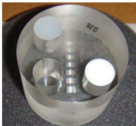
FIGURE 3.3.1. Example of a voxel density value phantom used for dental CBCT containing air, low-density polyethylene (LDPE), Teflon and acrylic inserts.
