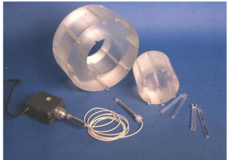
FIGURE A3.1. Left: Schematic image of a CTDI phantom, indicating central and peripheral holes for pencil ionization chamber measurements (Image from reference 61). Right: Pencil ionization chamber and standard CTDI phantoms for head (16 cm diameter) and body (32 cm diameter), respectively (Image from reference 82).
