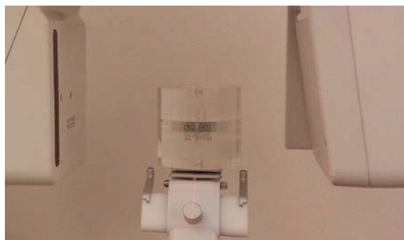
FIGURE 4.1.1. An example of the DIN phantom for acceptance tests (QUART DVTap) on the positioning aid (holder) of a dental CBCT system. Image courtesy of Chang Eui Lee and Ralph Schulze (Mannheim).
