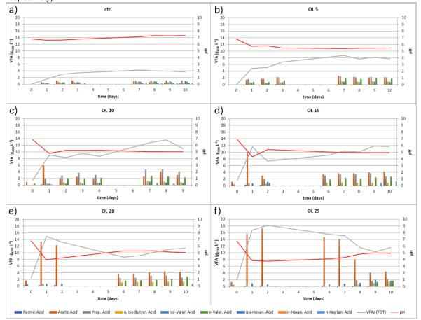
Figure 1, total VFAs production, VFAs characterization, and pH curve for each tested condition. a) control condition, b) OL 5, c) OL 10, d) OL 15, e) OL 20, and f) OL 25 kg<sub>TVS(mixture)</sub>  $m^{-3}$
